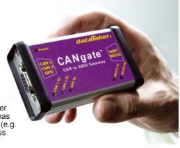
Two CAN interface ports are included, which allow connection of two independent CAN networks. *CANgate's* versatile configuration options allow you to select the parameters of interest, apply statistical functions (average, minimum, maximum) and control the format in which data are returned. *CANgate* supports widely used protocols such as ISO-15765 and SAE-J1939, as well as raw CAN frames.
