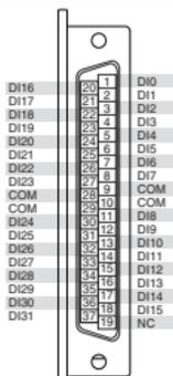
Each channel has a DI pin to which you can connect a digital input signal. The NI 9425E has four common pins, COM, that are internally connected to the isolated reference of the module.
