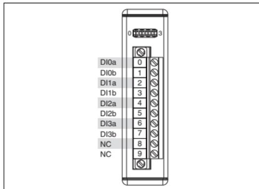
**Figure 2.** NI 9435 Terminal Assignments
