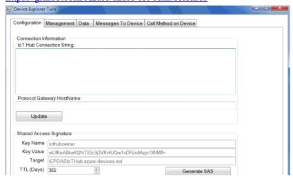
ii. Open and go to **Configuration** window, paste the **Connection String** of your IoT hub, and click the Update button, and then the Device Explorer connects to your IoT hub successfully
