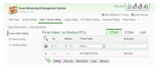
iv. Complete the settings, download the setting to PMC-5231, and then go to the "**Main Page**" to check the communication status with the power meter.
