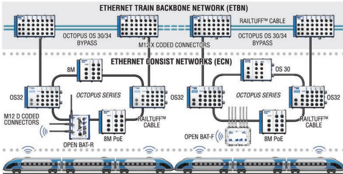
Figure 4: Ethernet Train Backbone Network
