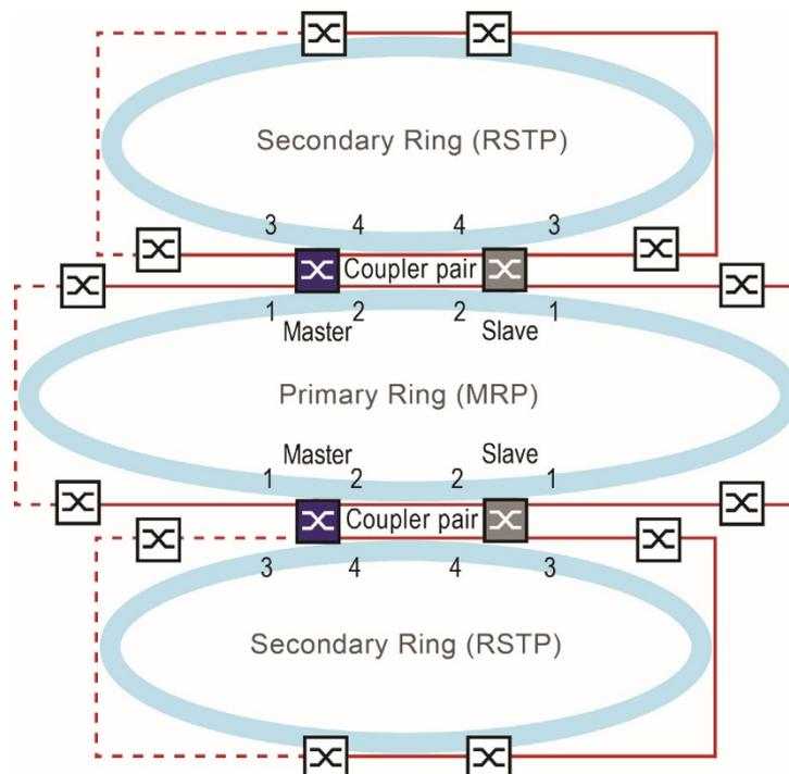
Figure 2: Coupling Redundant Rings
