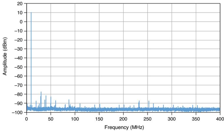
Figure 4. 1 MHz Spectrum<sup>[13]</sup> at 6.5 V<sub>pk-pk</sub>, Measured
