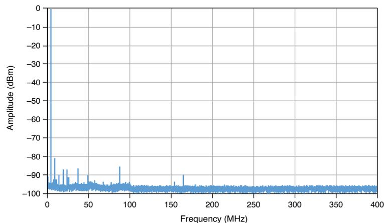
**Figure 3. 10 MHz Spectrum<sup>[13]</sup> at 2  $V_{pk-pk}$ , Measured**
